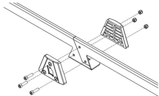
2. Loosely fasten the side rails using the M8 Bolts and channel nut. Refer to the diagram.
