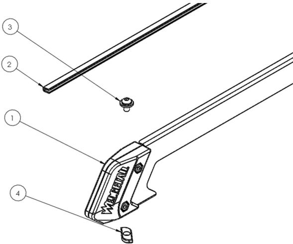
2. Fasten the Side Rails to the platform using M8 Stainless bolt and washers and channel nuts. Place the channel nuts in the cross bar and rotate 90 degrees to ensure secure fitment as shown.
