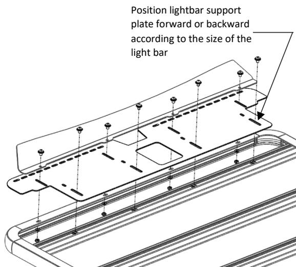
4. Once in the correct position tighten fasteners securely, check at frequent intervals.
