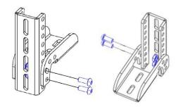
Mount awning bracket to WT platform as shown using M8 Bolts and channel nuts provided. Do not fully tighten.
