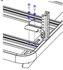
4. Put the bracket on the top of the platform and tighten the bolts.
