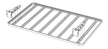
Loosely assemble the brace bracket using the M8X25 Hex Bolt and washer using the channel nuts.
