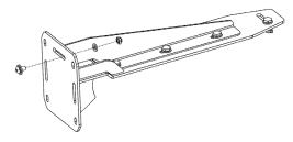
3. Assemble the bracket on the top of the cross bar using the bolt, washers, and channel nuts. Refer to the diagram.
